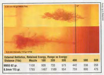
This photo illustrates the difference in performance between the M855, 5.56x45 NATO round (top) and the 6.8mm REM SPC using the Hornady bullet.
